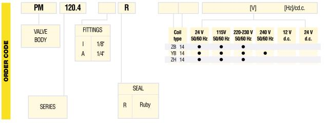
Note: Valve supplied with body (PM) and coil separate. Connectors to be ordered separately.
