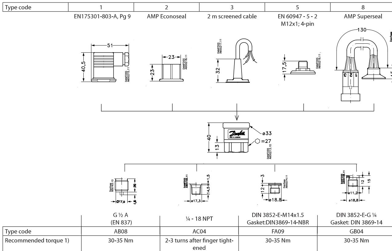
1)Depends of different parameters as packing material, mating material, thread lubrication and pressure level.
