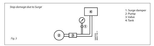
In cases where valves are closed momentarily, surges af a value in excess of that for which the pressure element is designed can occur. To avoid damage to the pressure element, a damping device should
