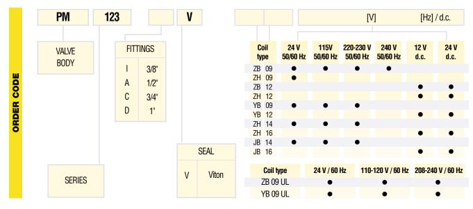
Note: Valve supplied with body (PM) and coil separate. Connector to be ordered separately.
